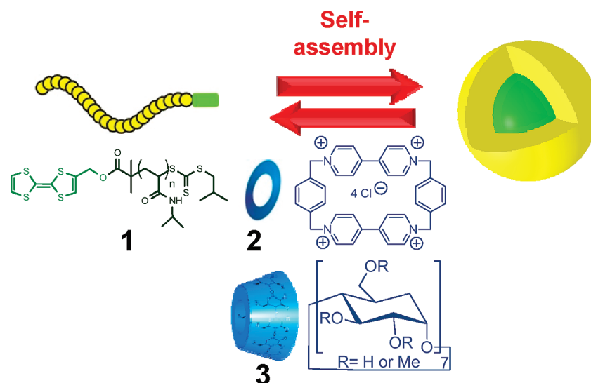
Figure 1. Schematic representation of the self-assembly of 1 and the structures of guests 2 and 3 used in this study.
